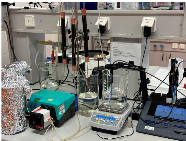
Fig. 1. Laboratory column tests of AOP with heterogeneous catalyst (magnetite)
