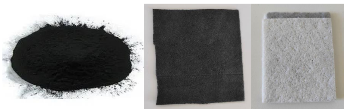
Fig. 1. Left – biochar 4073, centre – first prototype of textile filter, right – pilot textile filter.
