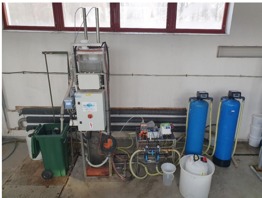
Fig. 2. Pilot technology for the quaternary treatment of filtered, biologically treated wastewater (composition from right to left) by combining the Fenton process with heterogeneous catalyst, the elimination of residual peroxide, biological treatment in the MBBR, and final sorption on activated carbon. Liberec WWTP
